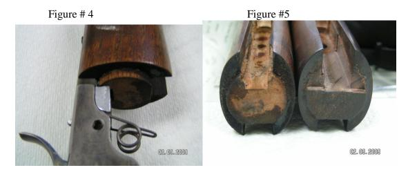
Remove the tang through screw and insert the unit into the stock. Use a scribe or sharp pencil to mark the area to be removed (see fig. #4) then, remove the excess wood all the way to the existing relief line. You can use whatever tools you have to trim the nose flat with the shoulder of the Butt Stock (see fig #5). A simple wood rasp will do it in about two minutes, a small fine toothed saw will take about the same time. Be careful! Some inletting may be necessary later to get the stock to fit.
