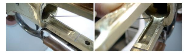
It's going to be necessary to remove a small amount of material from the area where the lower tang enters the receiver in order to allow the mounting base of the coil mainspring assembly to lie flat against the lower tang when installed.
