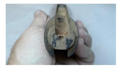
You will have to remove enough wood from the groove on the bottom of the stock to allow enough clearance for the coil mainspring conversion to move freely. A Dremmel tool with a drum sander works well for this. Wood will have to be removed from the front of the stock to the hole where the stock screw passes through.
