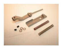
The Coil Mainspring Conversion Kit contains a strut assembly, two coil mainsprings (the red spring is 10% lighter than the other spring), a mounting base, three spring spacers, and two 6-40 setscrews.
