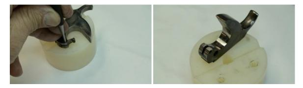
Next, remove the "T" strut from the hammer by tapping the pin out that holds it to the hammer. It would be a good idea to polish the surface of the inner curve on the back of the hammer. This is the surface that the bearings on the strut ride on. The polishing of this surface will provide a smoother feel to the action.
