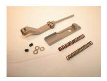
The Coil Mainspring Conversion Kit contains a strut assembly, two coil mainsprings (the red spring is 10% lighter than the other spring), a mounting base, three spring spacers, and two 6-40 setscrews.
