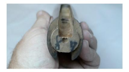
You will have to remove enough wood from the groove on the bottom of the stock to allow enough clearance for the coil mainspring conversion to move freely. A Dremmel tool with a drum sander works well for this. Wood will have to be removed from the back of the stock to the hole where the stock screw passes through.
