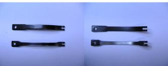
Here is what that mainspring looks like compared to a stock Uberti mainspring. Notice that the top surface of the spring is ground and sanded lengthwise. This removes the diagonal lines that are in the original spring. Doing this will eliminate the chance that one of those lines will develop into a crack.
