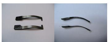
The photo on the left shows properly lightened lever/lifter arm springs. The photo on the right shows the thickness of these springs compared to a stock Uberti spring. Notice that the grinding and sanding lines run lengthwise on these springs, so they won't develop into cracks. When you do this, make sure that the little tips of the springs are smooth and round where they ride on the lever and lifter arm.
