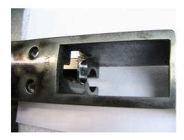
Have you ever had the last round that you just loaded sit crooked in the carrier and refuse to feed because the rim is catching on the frame as the carrier is trying to lift it up? A lot of you have called to ask what you can do to get that first round to feed more smoothly. I've coached so many of you on how to correct this issue that I thought I'd post some pictures of what this modification looks like.
